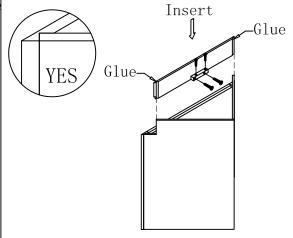
Step5:Install screws as shown.
