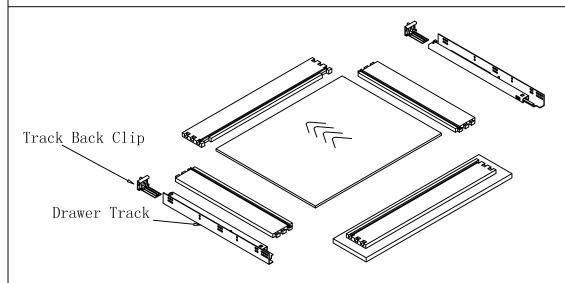
Step1:Install sides on drawer front.Tap with hammer if needed to make flush.
