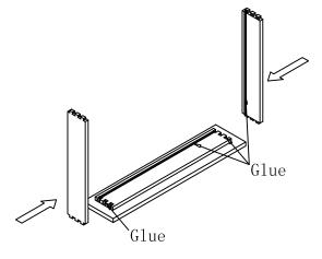
Step3:Install back of drawer by spreading the sides of drawer just enough to allow back of drawer to be locked in.As before, glue dovetail joints.
