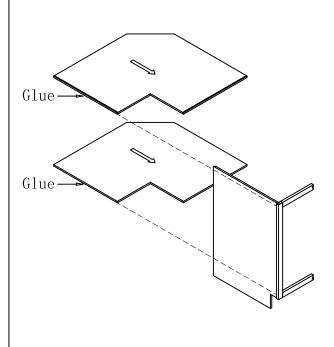
Step3:Slide side panel into hook grove on top and bottom.carefully si ace frame past each other. Install screw into face frame.
