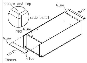
Step5:Install screws into cabinet .Slide toe kick backer into cabinet grove.
