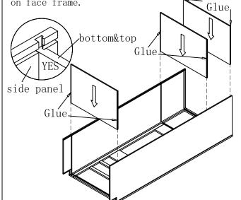
Step3:Slide Back Panel into slot and make sure that panel lines up flush
