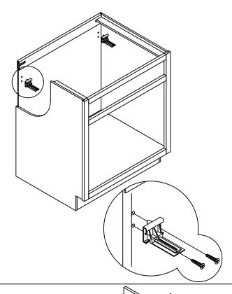
Step3:Slide tracks back and line up front track holes with faceframe hole and screw in.
