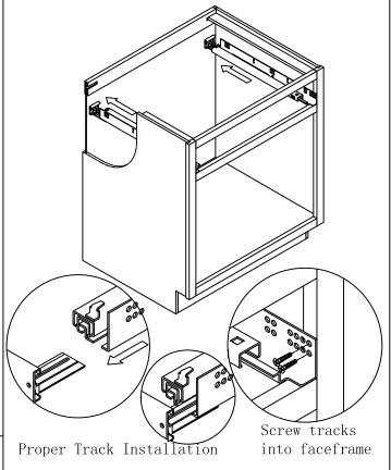
Step4:Slide drawer into cabinet making sure that back of drawer locks into metal tab at end of track. You should hear the track click into place when it locks in Open and close drawer to make sure of proper operation. Adjust drawer face with front clip adjustments as needed
