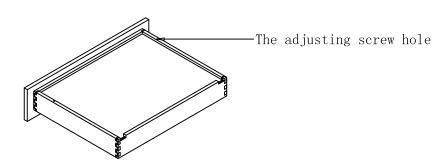
Step2:Install track mounting clips secure with supplied screws
