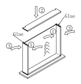
Step2:Slide plywood bottom into grove on drawer sides. No glue here to allow for natural expantion and contraction of drawers.
