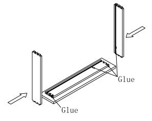
Step3:Install back of drawer by spreading the sides of drawer just enough to allow back of drawer to be locked in. As before, glue dovetail joints.
