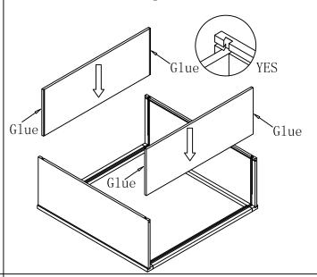
Step3:Slide Back Panel into slot and make sure that panel lines up flush with top and bottom.
