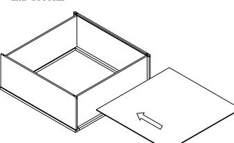
Step4:Install hanging rails top and bottom. Make sure all rails are flush with side panels.
