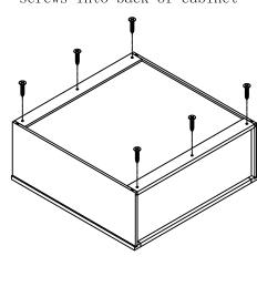
Step6:If Width is 30" or over, install screw blocks at face frame on top and bottom.
