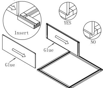
Step2:Slide Top and Bottom into hook grove in sides of the cabinet. Make sure that bottom of Floor is seated into grove on back frame
