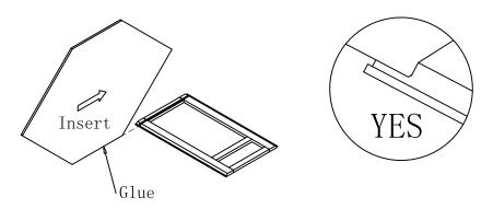
Step2:Slide side panels into hook grove on bottom.
