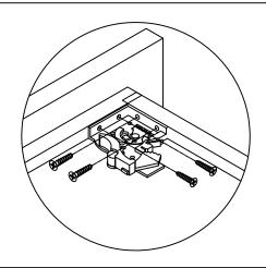
Step2:Install track mounting clips secure with supplied screws
