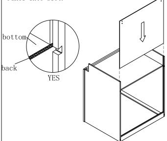
Step2:Slide I-Beams into slot of side panel till they lock into grove in Face Frame.
