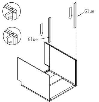
Step3:①Lightly push side panels apart ②to allow hanging rail ③to lock into grove on end panels
