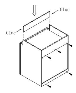
Step8:this is an adjustable shelf install as need with your oven, Install the screws into wood blocks on the face frame and side panel and back panel.
